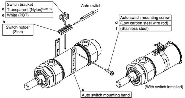
\* Band (c) is mounted so that the projected part is on the internal side (contact side with the tube).
