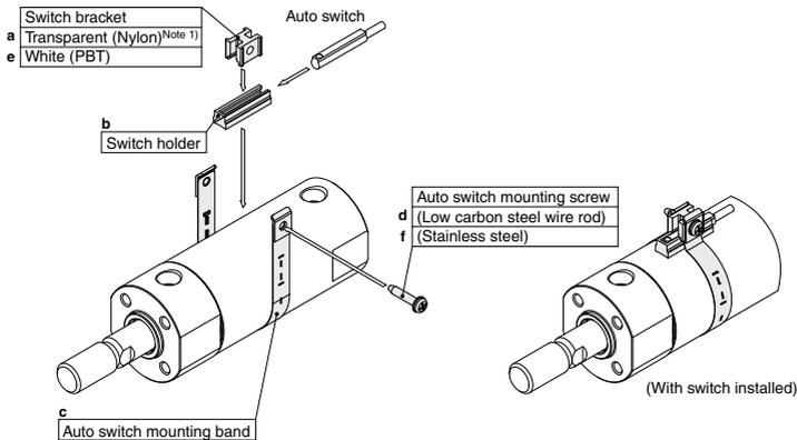
\* Band (c) is mounted so that the projected part is on the internal side (contact side with the tube).
