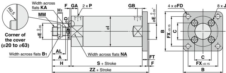
\* End boss is machined on the flange for  $\phi E$ .
