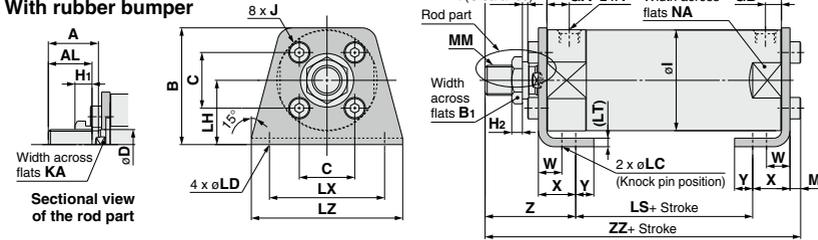
\*1 The rod end nut should be mounted in the position t (clearance) so that it will have a clearance of 1 mm or more in order to prevent interference of the nut with the bolt for mounting bracket when the rod is retracted.
