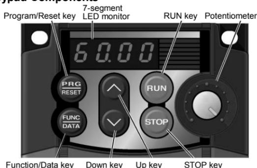
Table 3.1 Names and Functions of Keypad Components
